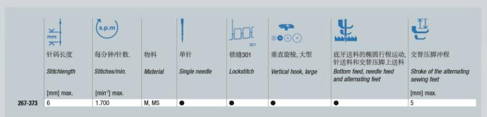
● = 标配缝制配件 / Standard equipment M = 中等厚度材料 / Medium-weight material MS = 中等厚度至厚重材料 / Medium-weight to heavy-weight material
